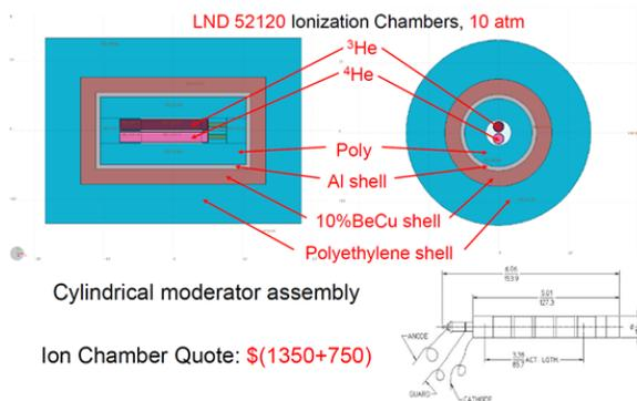
The novel design (U.S. patent pending), modeled in FLUKA, includes the new type of neutron moderator with the layer of beryllium copper material improving and equalizing the dose rate response to higher energy neutrons, and the new type of neutron-sensitive element made of the two small ion chambers, filled with <sup>3</sup>He and <sup>4</sup>He gas at the same pressure.
