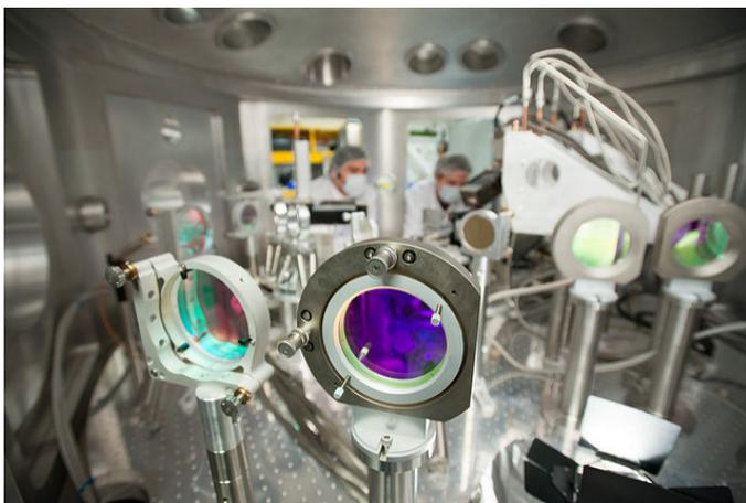
This high-intensity laser is focused onto targets (gas, liquid, and solid) and used to study warm and hot dense matter, high pressure science, and even the insides of giant gas planets like Jupiter. It can also be used as a driver for generating mono-energetic beams of proton (and other ion) beams and for accelerating electrons to hundreds and even thousands of MeV.
