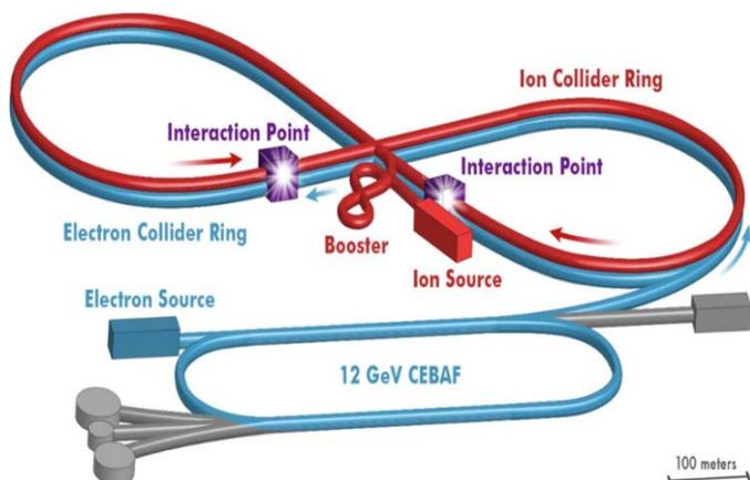
Figure 2: Schematic layout of the envisioned JLEIC accelerator complex.
